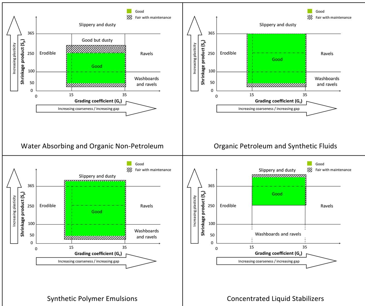
**Figure 30: Expected Performance of Unpaved Roads after Chemical Treatment.**
