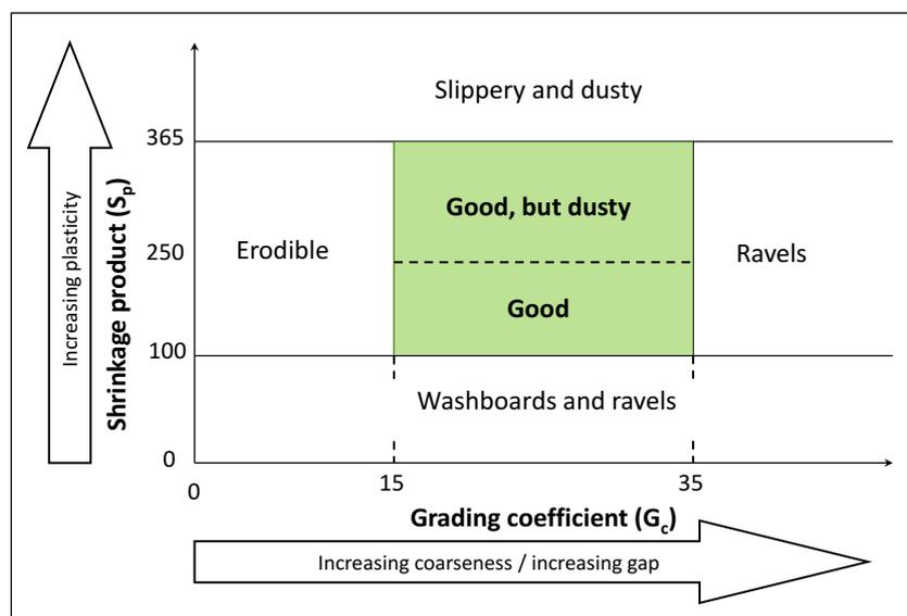
**Figure 27: Material performance predictor chart (adapted from Paige-Green, 1989)**
