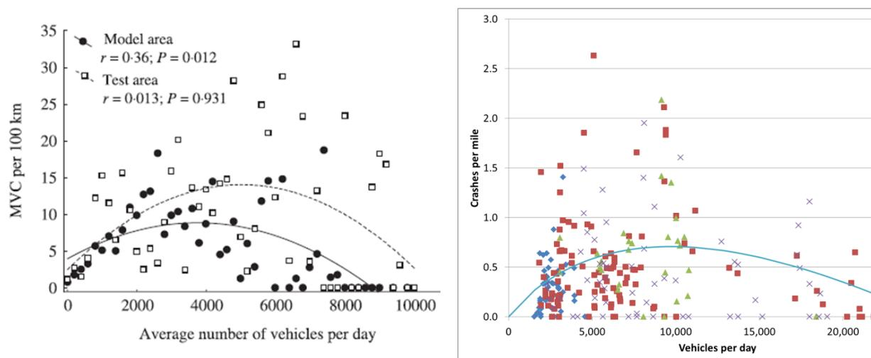
**Figure 12: Average Animal Vehicle Collisions for Road Segments of Different Traffic Intensity. Left: Moose in Sweden (Seiler, 2005); Right White-tailed Deer in North America (Dezort and McGowen, 2010)**
