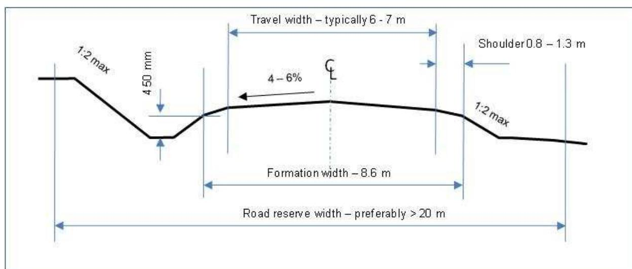
**Figure 29: Cross section of a well-constructed gravel road (recreated from Republic of South Africa Department of Transport 2009).**
