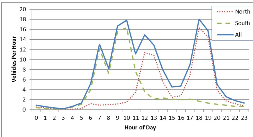
**Figure 9: Average Daily Traffic Distribution on Oyu Tolgoi Road (Unpublished Data Provided by Oyu Tolgoi Mine Dec. 2014 – June 2015)**
