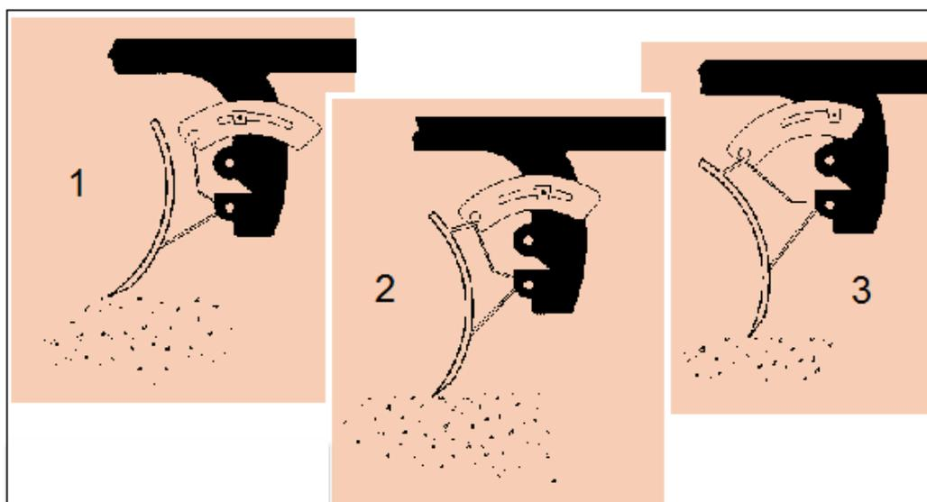
**Figure 28: Examples of how the tilt, or pitch, of the cutting blade can be modified to achieve varying results (Skorseth and Selim, 2000).**
