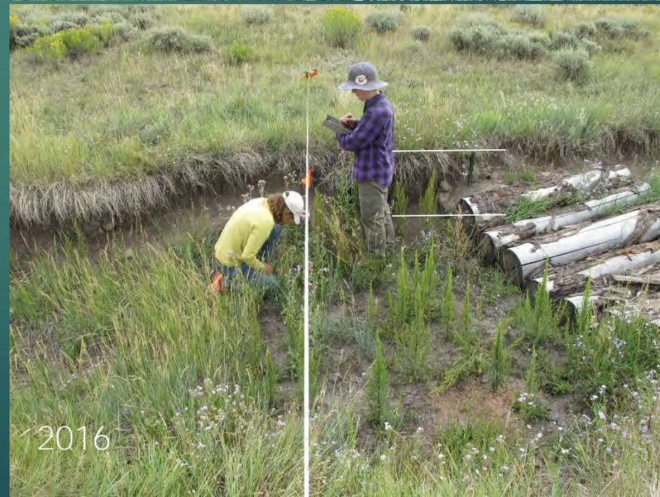
Notice the location of Gay's waist compared to the bank; approximately 1' of sediment was deposited, due to the log structure
