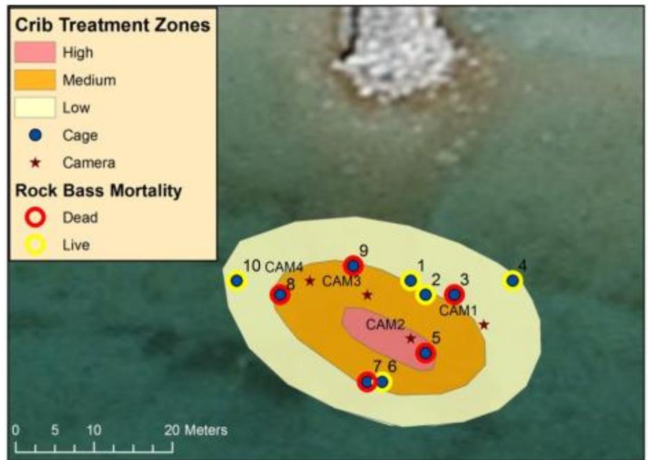
Figure 3.5. Treatment cages where Rock Bass had died within 24 hours of treatment are shown with red circles. Camera 2, which was placed within the high treatment zone, shattered approximately 15 minutes into the treatment due to the pressure from the seismic treatment.
