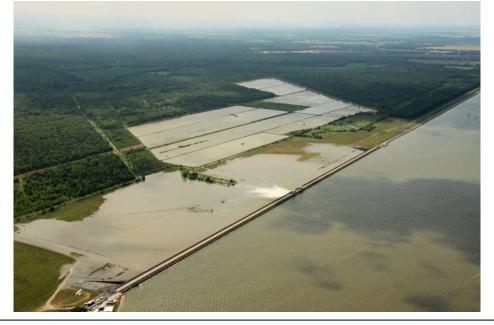
**Figure 8.** The Morganza Spillway (long line in center) during the 2011 Mississippi Flood. The Morganza Spillway was opened during this flood, allowing the Mississippi River, on right, to begin to flow into the Morganza Floodway (fields and forests on the left). © NASA
