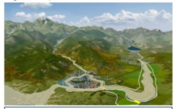
Flood management with green infrastructure during a moderate flood (e.g., 1 in 10 year frequency). In many locations floodwaters are not directly adjacent to levees. The bypass is in use; greater extent of inundated floodplain habitat.
