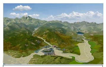
Traditional flood management during a large flood (e.g., 1 in 100 year frequency), levee breaches lead to urban flooding and unplanned flooding of agricultural land.
