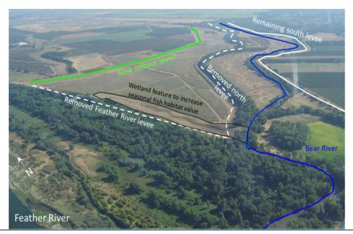
**Figure 7.** A setback levee project on the Bear River at its confluence with the Feather River (Central Valley, California, USA). To increase conveyance and reduce backwater flooding, the north levee of the Bear and a section of levee along the Feather River were removed (white dashed line) and two-mile long setback levee was built (green line). The project lowers flood risk along the Bear and restored hundreds of acres of floodplain habitat. Figure adapted from Williams et al 2009
