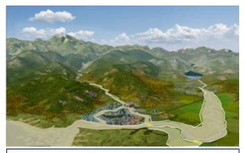
Flood management with green infrastructure during a large flood (e.g., 1 in 100 year frequency). Both bypass and flood detention area are in use. Agricultural land is flooded but primarily land planned to flood; either in flood-compatible crops or with compensation mechanism.
