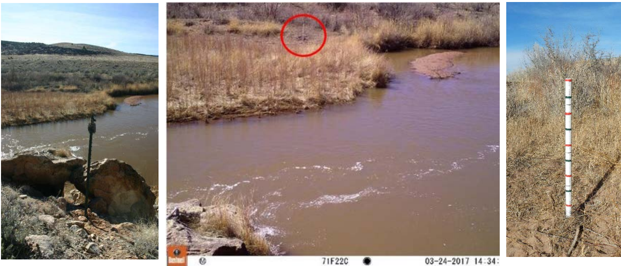
Figure 43. Installation of staff gage and wildlife camera at the Slickrock Upstream site in March 2017. From left to right: installed camera, shot from camera at time of installation (staff gage circled in red), and staff gage close-up (post-release).
