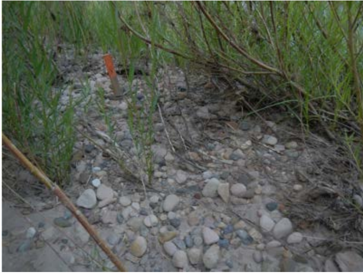
Figure 39. Bedrock erosion stake monitoring, a close-up view of stake #1 post-release. The bare wood below the blaze orange is the depth of scour.
