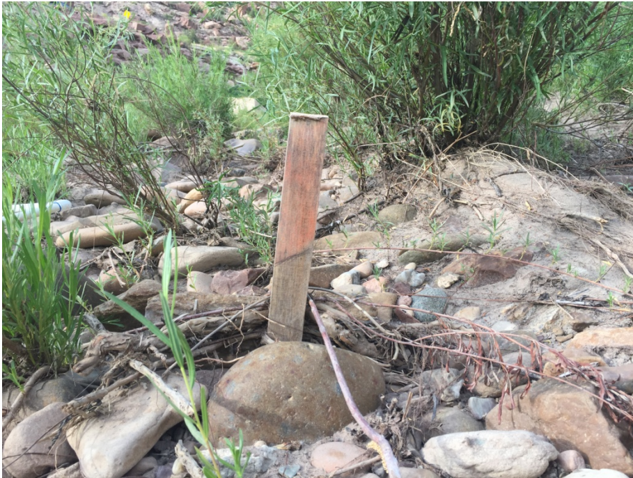
Figure 27. Post-release scour on low floodplain at Slickrock Downstream site. Stake painted to depth installed pre-release (3/22/17). Approximately 0.5 feet of material was scoured from this location.
