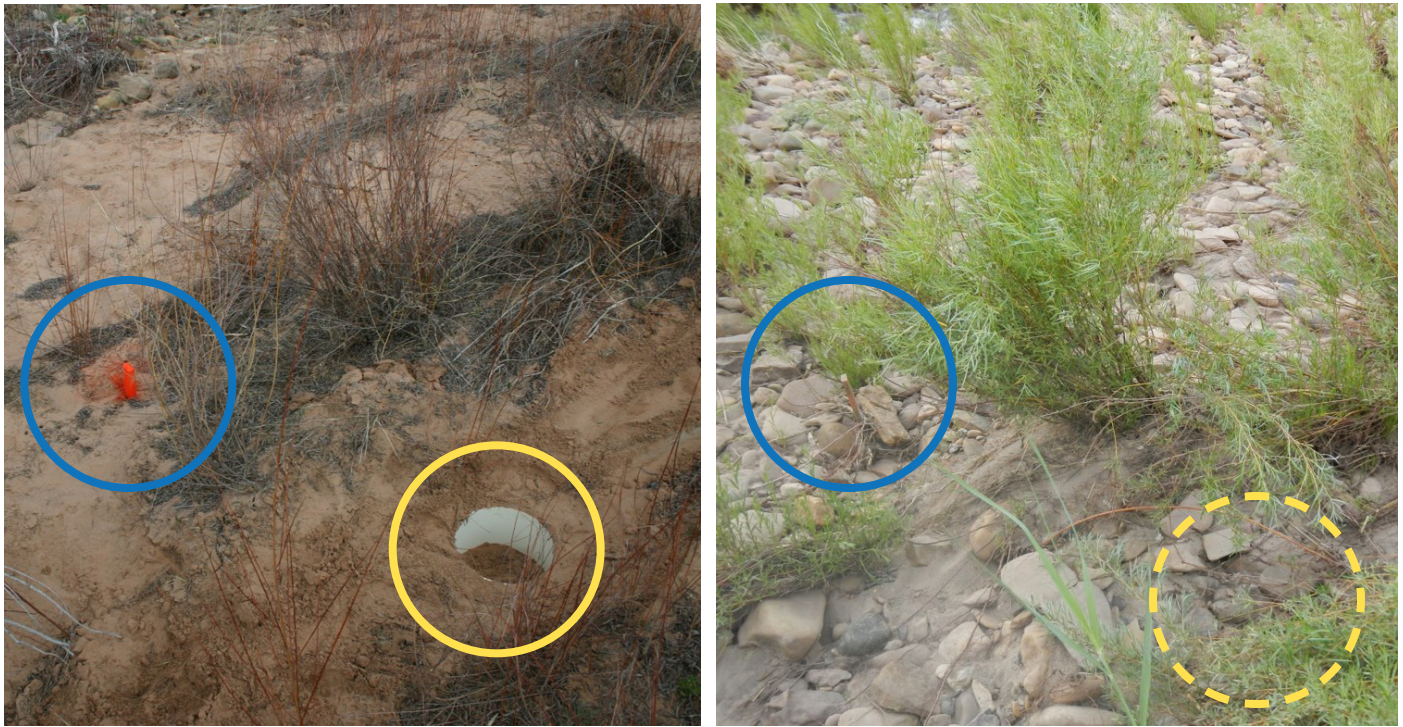
Figure 3. Slickrock Downstream sediment trap (yellow circle) and erosion stake (blue circle); pre-release photo on left (3/22/17), and post-release photo on right (7/6/17). Note the scouring of fine material observed with the orange erosion stake between pre- and post-release. It is estimated that the sediment trap was washed away with strong scouring flows during the managed release (absence of sediment trap post-release).
