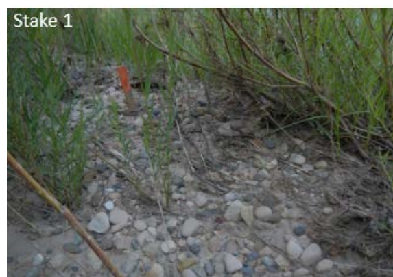
Figure 60. Point bar at Bedrock Site, close-up of sediment scouring (Erosion stake #1, river left), pre-release 3/23/17 on left, and post-release 7/8/17 on right.
