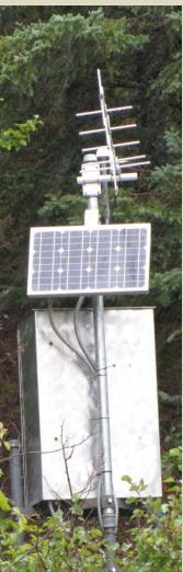
USGS Gaging Station with solar powered satellite transmitter for real time data collection and transfer.
