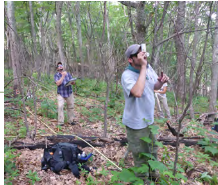
Estimating canopy cover using a densitometer in the Warm Springs Mountain Restoration Project. Photo: Nikole Swaney/TNC
