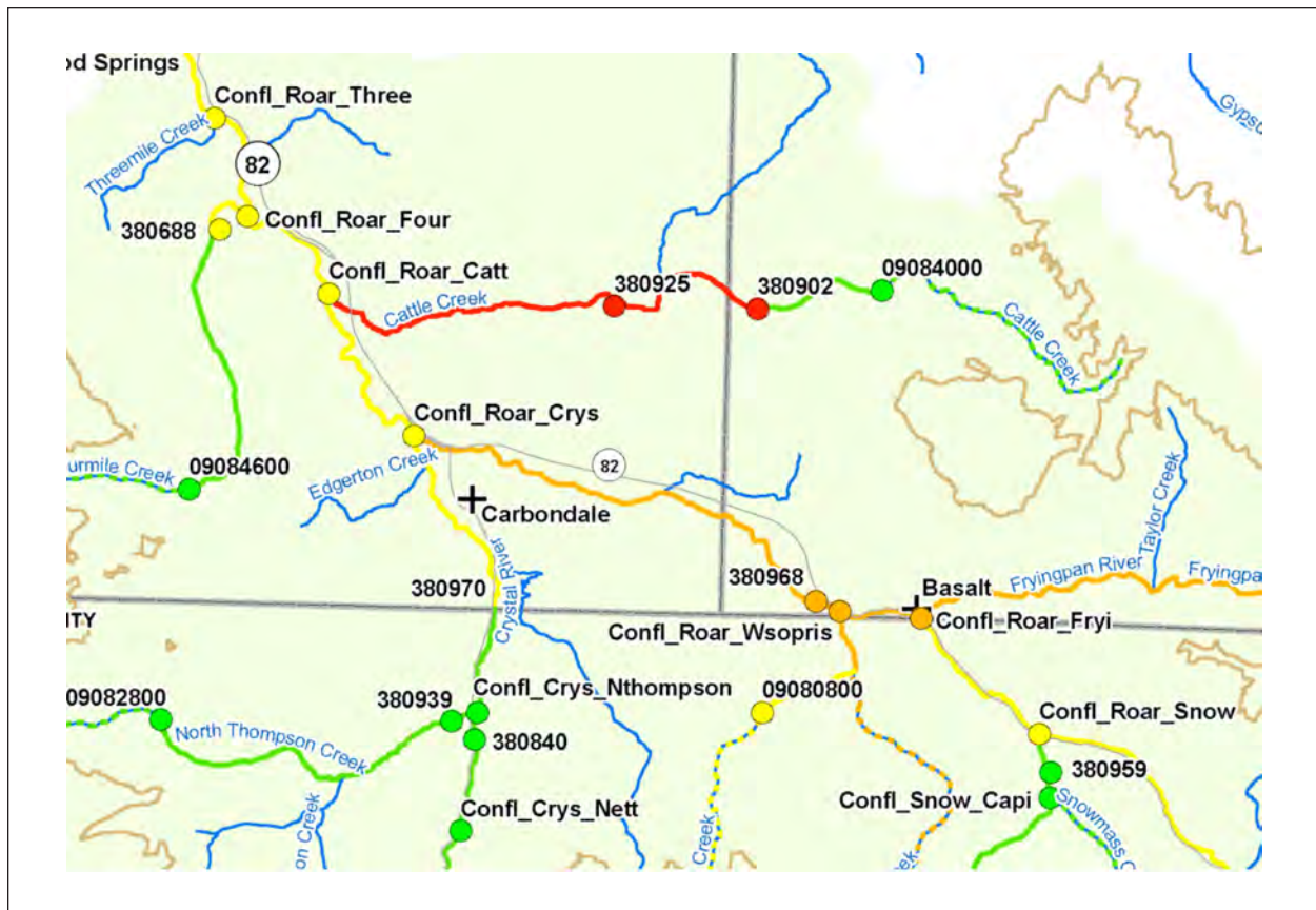
Figure 2. Watershed Flow Evaluation Tool output detail, showing level of flow-related ecological risk for each river reach. Risk levels: red = high, orange = moderate, yellow = minimal, green = low. Blue = not modelled (no flow data).
