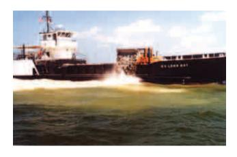
NC DMF vessel deploys riprap marl to restoration site. © NC DMF
