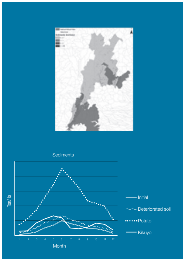
Figure 6. SWAT Model: Estimation of sediments in Bogota's water supply systems, Colombia. Bogota Water Fund. • Source: CIAT, 2007, Study hired by TNC, Bogota Water Company (EAAB) Patrimonio Natural & Parques Nacionales.
