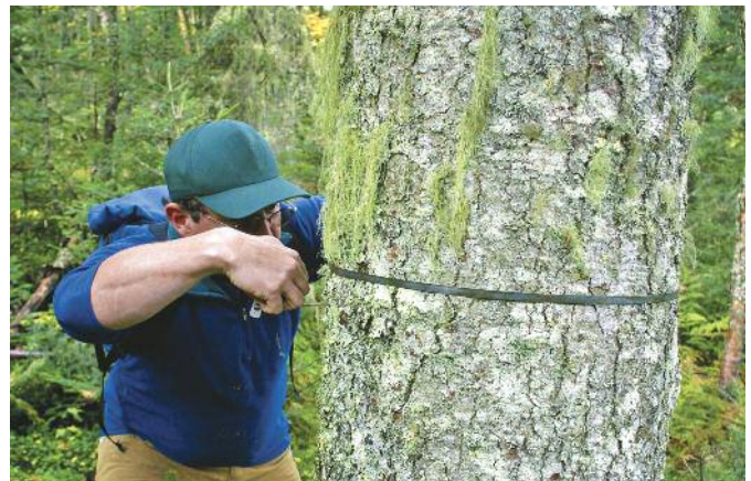
Double-checking ground measurements of dbh is a standard part of the verification process. Photo Credit: © Eric Aldrich/TNC
