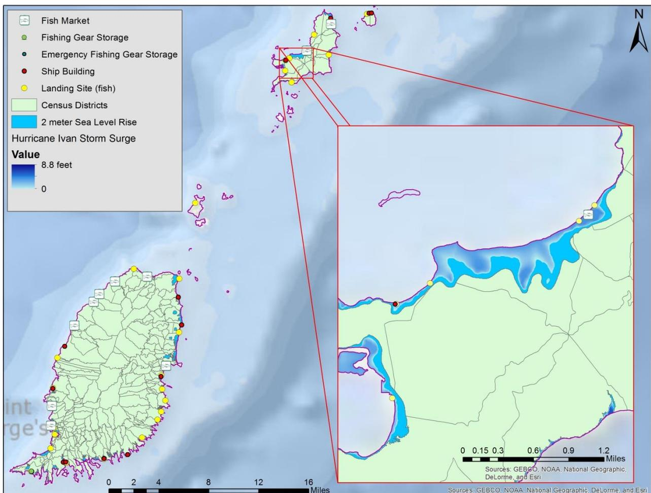
FIGURE 2 LOCATION OF FISHERIES FACILITIES AND EXTENT OF FLOODING FROM A MODELED TWO-METER SEA LEVEL RISE AND STORM SURGE FROM A HURRICANE IVAN TYPE STORM. INSET DETAILS MODELED EXTENT OF FLOODING FOR WESTERN CARRIACOU.
