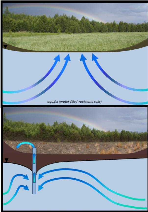
The following schematics illustrate this concept for a groundwater-dependent wetland, where a pumping well is installed to draw water from a wetland.
