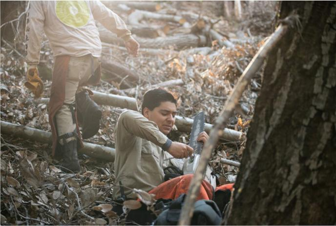
Nico Costillas adjusts the chain tension on the AMLT chainsaw he uses. Maintaining and adjusting tools is part of in-depth knowledge of the work, ensuring safe working conditions.
