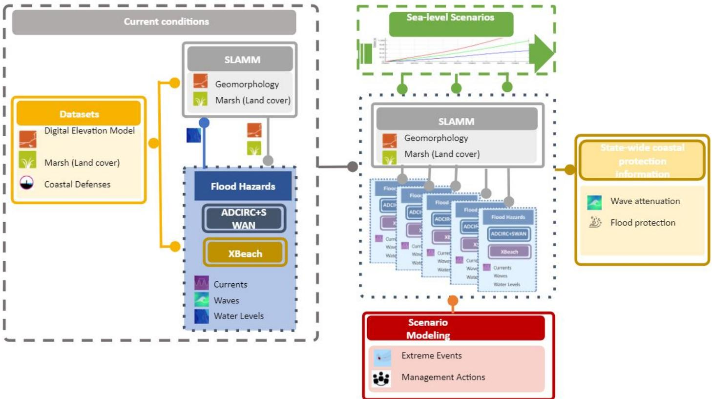
Figure 2. Depiction of the modeling framework being used to estimate the wave attenuation capacity of natural and nature-based features across Maryland.
